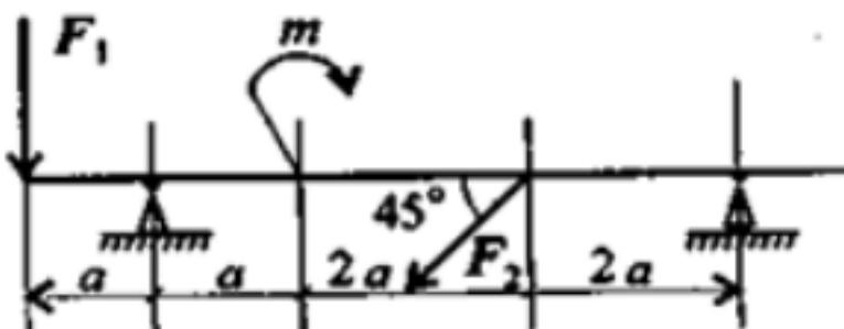
$$F_1 = 18 \text{ kN}; F_2 = 7 \text{ kN}; m = 10 \text{ kN}\cdot\text{m}; a = 0.3 \text{ m}$$
