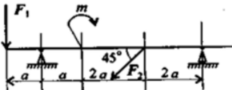
$$F_1 = 18\text{kH}; F_2 = 7\text{kH}; m = 10\text{Kn}\cdot\text{m}; a = 0.3\text{m}$$
